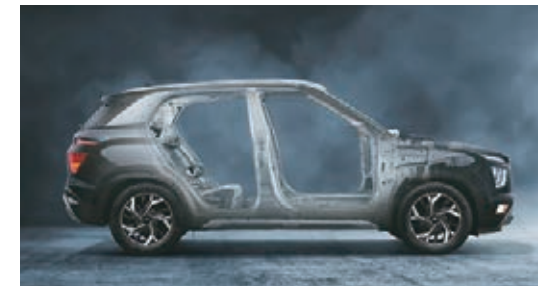
Strong body structure with AHSS
